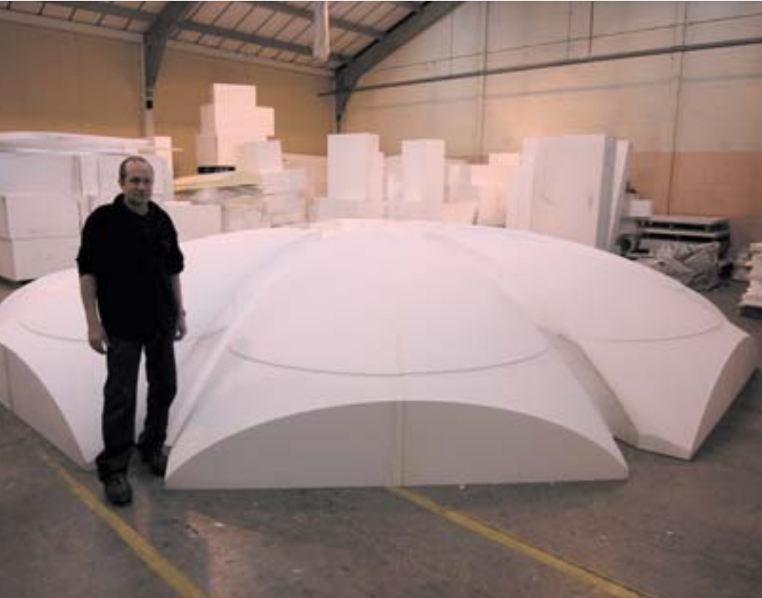
This massive octagonal template was used to form a vaulted stonework arch.
